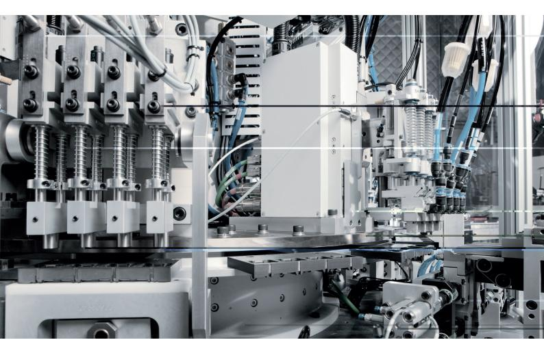
The direct drive rotary table is freely programmable and allows the shortest indexing times at the highest precision.
